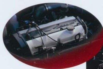
Left: ZX2 16-valve Zetec engine. Below: Sedan/Wagon 2.0L engine.
