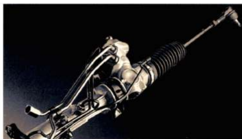
Power rack-and-pinion steering improves steering response.
