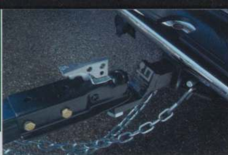
7-wire trailer wiring harness and frame-mounted hitch receiver (shown with aftermarket hitch equipment).
